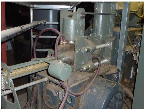
Fig. 15: Pressing cylinder
