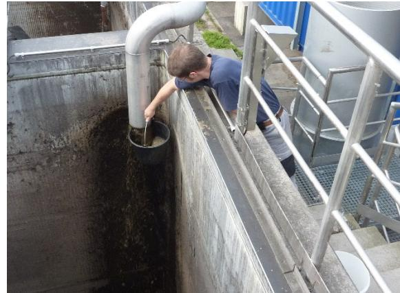
Fig. 18: Sampling of press fluid
