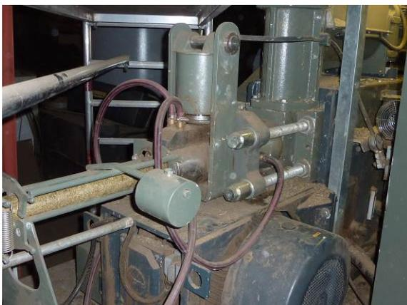
Fig. 15: Pressing cylinder
