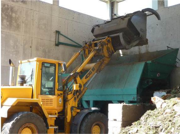
Fig. 5: Loading of the dosing feeder
