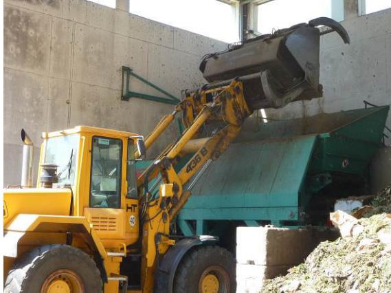
Fig. 5: Loading of the dosing feeder
