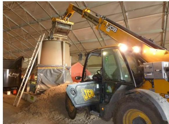
Fig. 14: Loading of the briquetting unit
